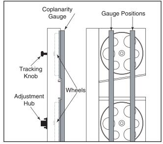
Figure 63. Checking for coplanarity.
